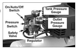
Safety Valve: If the pressure switch does not shut off the air compressor at its "cut-out" pressure setting, the safety valve will protect against high pressure by "popping out" at its factory set pressure (slightly higher than the pressure switch "cut-out" setting).
